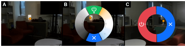
Figure 8: A: The user invokes an Radi-Eye interface for appliance control by gaze dwelling on an appliance. B-C: The object-dependent interface adapts to the selected appliance (B: lamp, C: fan) and is centred around the user's head.
