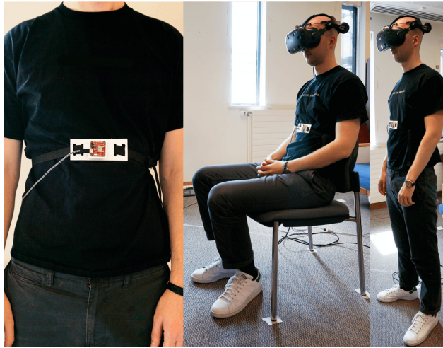
Fig. 2. Set-up of the experiment and each posture. Left: The IMU attached to the participant’s torso. Middle: The participant is seated on a non-swivel chair in seated posture. Right: The participant stands in a natural position when in the standing posture.
