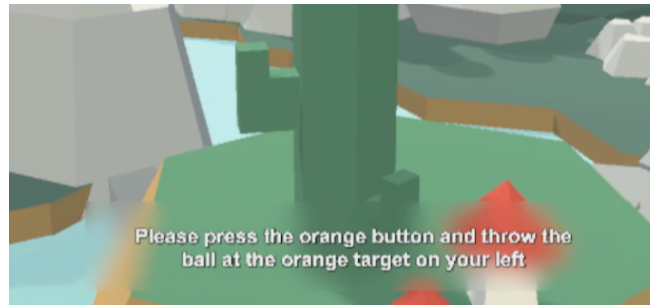
Figure 2: Background Blur blurs the background behind the subtitles when the user is gazing on the subtitles.
